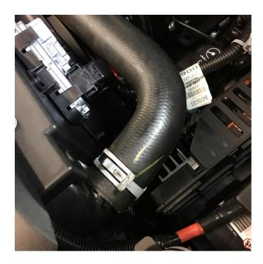
After it is separated, the hose can be pushed back against the radiator and the clamp returned to its normal position. Check the backside of the hose for clearance to the clutch. If necessary, create more clearance in this way as needed.
