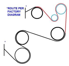
**Diagram 2** - Alternate belt routing for 2011-present models that need clearance around the power steering reservoir. This routing is slightly longer than Diagram 1, so the same belt length will be effectively looser.
