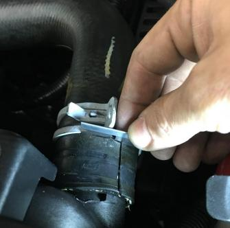
On 2011-Present models, remove tension from the upper radiator hose clamp and slide it to the end of the radiator neck underneath. Using the clamp as a guide, split the hose perpendicularly, then trace the circumference. You'll be removing approximately 1.25" of the hose end.
