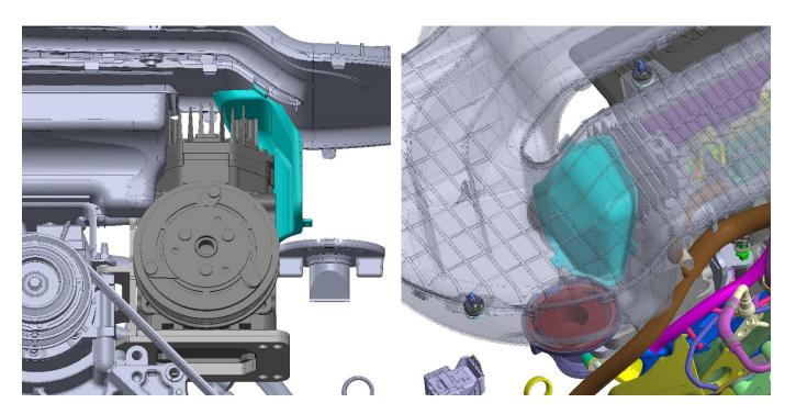
**2017-2019 continued:** Examples of how the included plenum patch part fits with the compressor. In the case of the SLM compressor, the head be milled to provide extra clearance for the filter and hose. Be sure to install the fittings and hoses facing the rear, as shown in **Steps 25 and 26**.
