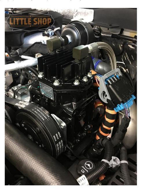
There are multiple positions in which the compressor can be mounted based on your application. If space allows, vertical mounting is preferred for the least amount of oil bypass. **SLM compressors can only be mounted vertically**. Please refer to the chart below to determine which position is to be used. These instructions describe the vertical mounting. Please refer to the 2000-2007 Classic instructions for horizontal mounting.
