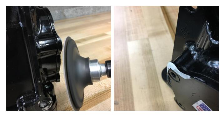
On the compressor body, lightly sand the corner of the rear cover plate as shown. This is to make clearance to the orange EGR electrical plug.
