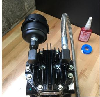
**SLM compressors:** Both ports will get the included 3/8 NPT elbows using PTFE tape or Loctite 545 sealant. The suction port (labeled with an "S" on top of the passenger side) will get an additional 3/8 adapter and then the included filter/silencer. The discharge port (driver side) will get the included leader hose threaded into the elbow. For heads that have been milled for flush fittings, the top will not be labeled. In this case, the same orientation described above should be used.
